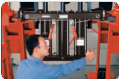
Swing Air-Jack, 133-83-1 9,000 lb. (4082 kg) Capacity
