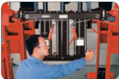
Swing Air-Jack, 133-83-1 9,000 lb. (4082 kg) Capacity
